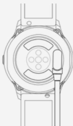
\*Only charge the watch in the way shown. Incorrect charging may damage the watch. Be aware that the two contacts of the USB cable are not allowed to contact the conductor at the same time, or it will cause the circuit to burn.
